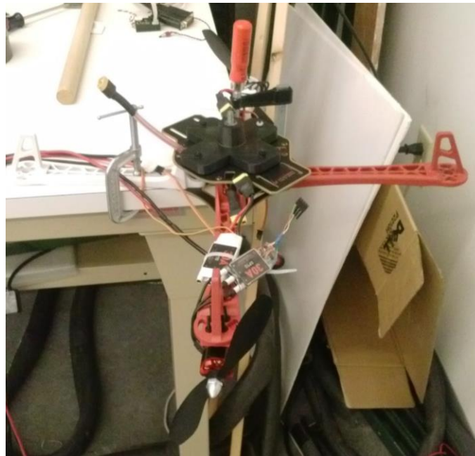
FIGURE 23: TEST SETUP FOR THE MOTOR SPEED
