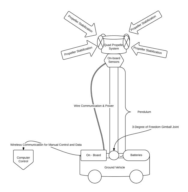
The system consists of a robot at the base with a long, light material stick connected to the top by a gimbal joint. This allows free motion for a quadcopter at the top which theoretically should be able to stabilize itself to be at a constant positioning above the robot.
